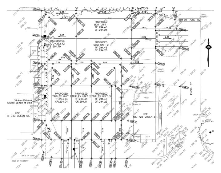
A storm sewer is available to the site on the Queen Street curb line. Surface water swales suggested along side and rear lot lines will direct flow to a catch basin proposed west of the street townhouses. Grading can contain surface water on proposed lots to prevent flow on to adjacent private property and minimize flow on to Queen or Enoch Street. The catch basin will collect surface water to convey it by underground lateral connection to the Queen Street storm sewer.
